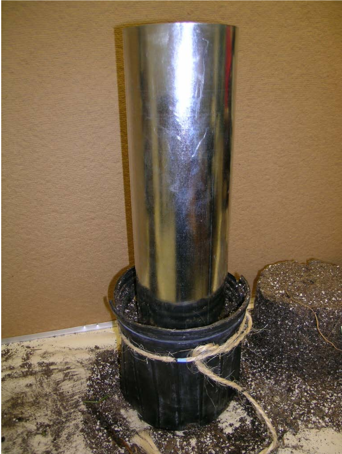
Figure 3. Removal of core section of soil from container.
