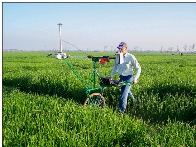
Kansas State University student and Phenocart developer Jared Crain collects data using the Phenocart in drought stress wheat trials at the Norman E. Borlaug Research Station, Cd. Obregon, Mexico.
