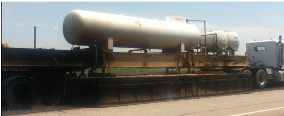
Figure 1-4 Heating and recycling unit in HIR train
