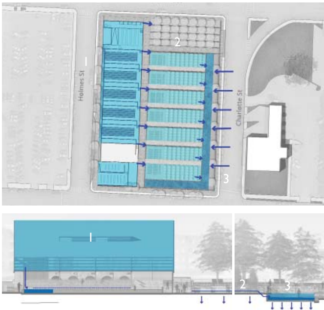
Figure 6.16 Water Capture | buildings (1) collect water to be used for irrigation (2) while the site is mostly permeable to collect and infiltrate rain water. The bioswale capture from the site and street (3) (KCDC 2016).
