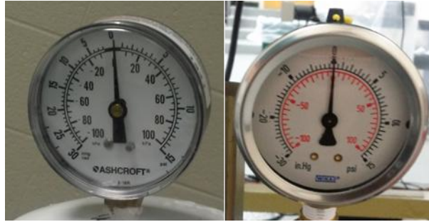
Figure E.1 Dry Ashcroft (left) and liquid-filled Wika (right) pressure gauges.
