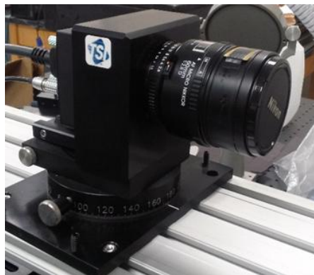
Figure A.1 PIV camera shown with 60 mm lens.
