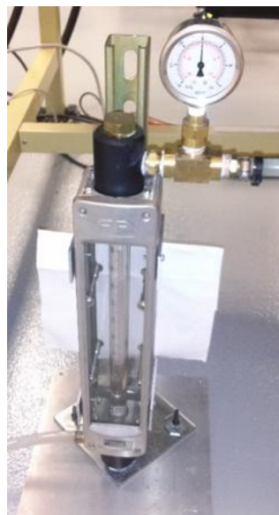
Figure E.4 Rotameter with attached liquid-filled pressure gauge.
