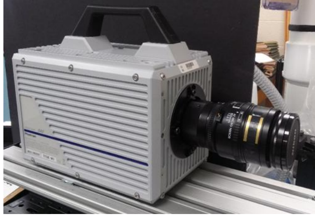
Figure B.1 High-speed digital camera. Shown with 60 mm lens.
