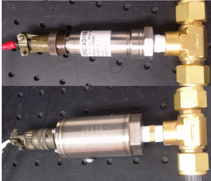
Figure E.3 Omega (top) and Viatran (bottom) pressure transducers.
