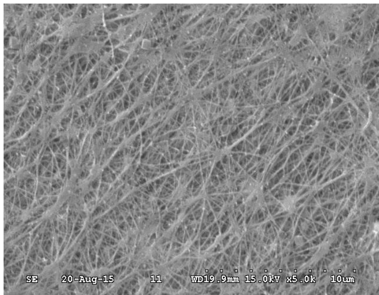
Figure A-1 - Ru loaded ePTFE membrane example 1 (top view).
