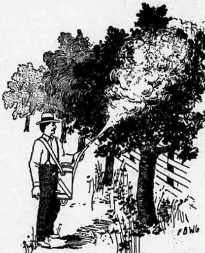
RIPPLEY'S COMPRESSED AIR SPRAYER WHITEWASHING MACHINE
