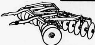
Seven-foot tandem disk harrow
