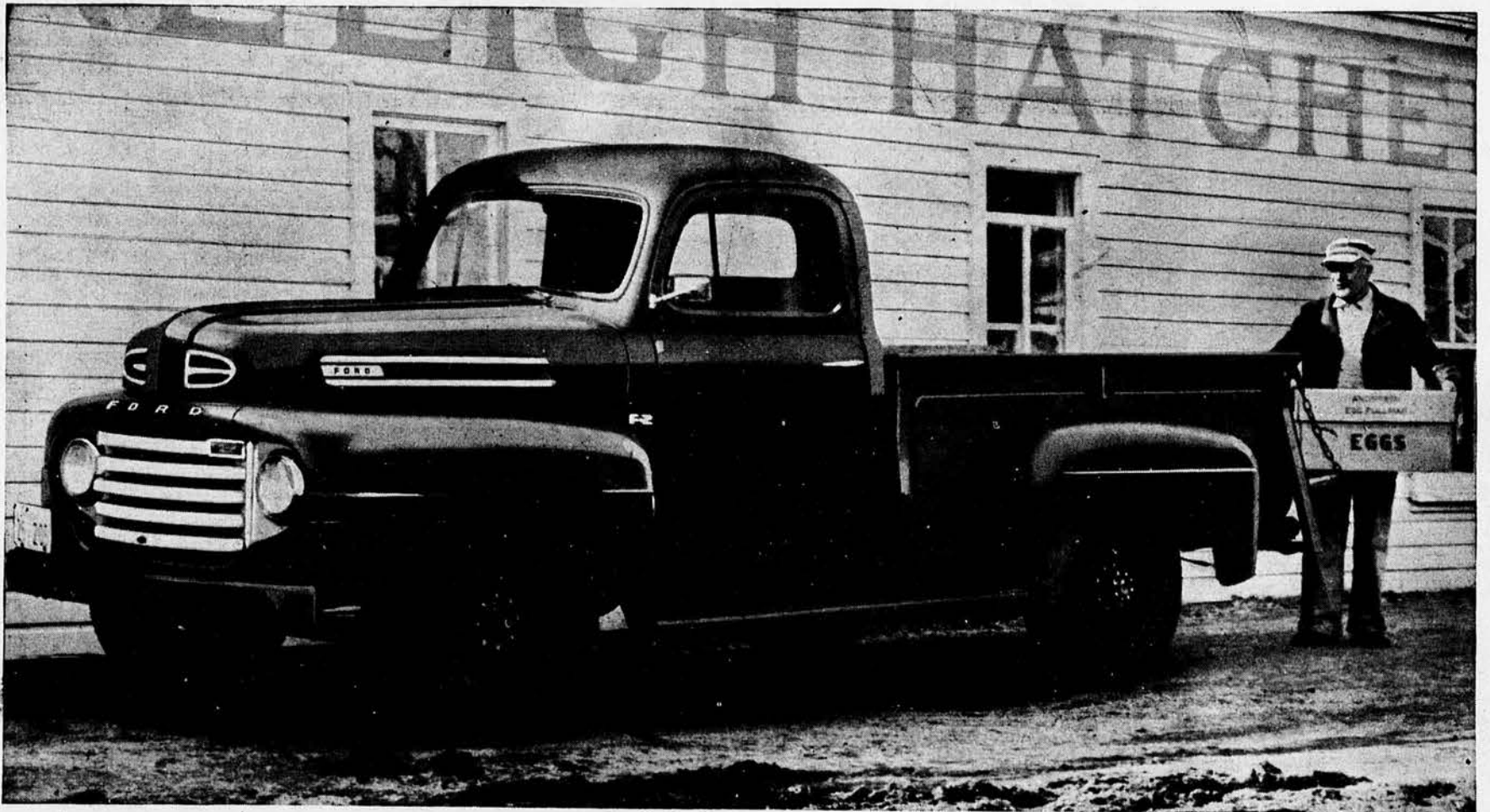
6-cylinder Ford Model F-2 shown has an 8-ft. Express Body mounted on a 122-inch wheelbase.
