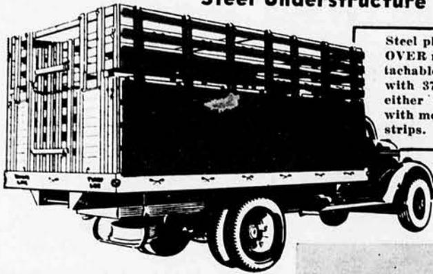
Steel platform FOLD-OVER model. Non-detachable 28" stock rack with 37" grain sides, either solid sides or with metal ventilating strips.
