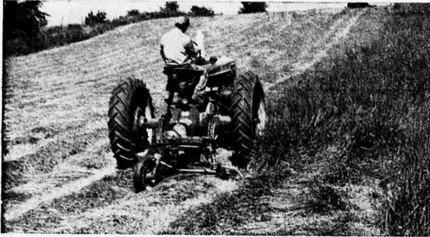
Win the race against weather. Mow 4 acres an hour with the McCormick semi-mounted tractor mower. Among its many advantages are V-belt drive for trouble-free, smooth operation; easy square corners without knocking down hay; safety cutterbar breakaway to prevent damage; and optional hydraulic lift. It fits most tractors. Attached to the drawbar in minutes.
