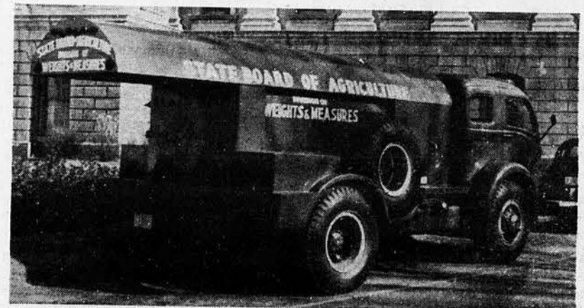
New, heavy-duty scale testing truck recently put in operation by the Weights and Measures Division of the Board of Agriculture. It features a special hydraulic lifting attachment and body designed to handle the eighteen 1,000-pound weights used in scale tests.
