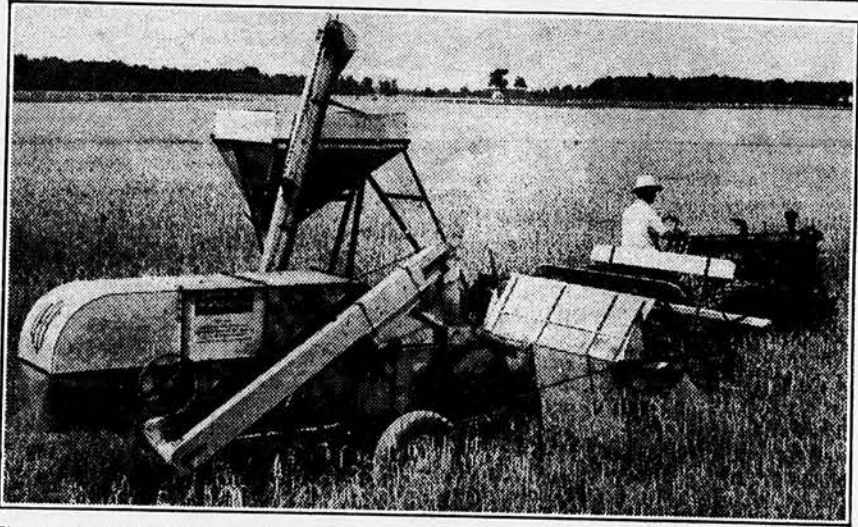
Five and 6-foot combines are increasing in popularity. Their first job is wheat harvest, as seen here, then the spring grains, followed by profitable off-season jobs such as combining Sweet clover, milo, grass seed; stationary threshing of alfalfa, and sorghum topping.
