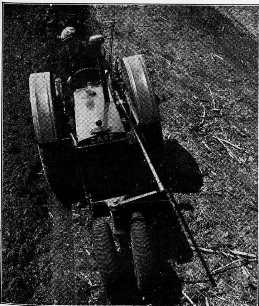
A new Case tractor—rubber tires and everything—plowing for spring planting. Farmers who use rubber tires report excellent service, less wear-and-tear on machinery and operator.
