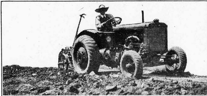
A tractor equipped with Firestone low-pressure tractor tires, plowed 5 miles in an hour on the Wisconsin state fair ground the other day, then was unhitched and made a speed record of 35.4 miles an hour. Which means that with low-pressure tires and new tractor models, a farmer may unhitch in the field, back up to a trailer and haul produce to market as fast as trucks, without hindering traffic. The Wisconsin tractor was designed by Allis-Chalmers and did nearly 5½ miles better than was expected of it in speed, altho that is about six times faster than tractors have been able to travel heretofore
