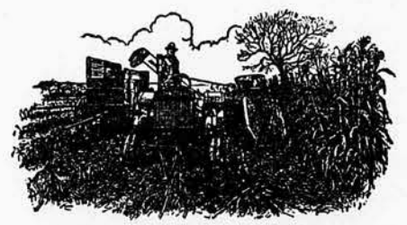
Pulling the corn picker and operating it with power take-off—a fast-working one-man equipment.
