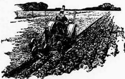
Makes a standard two-bottom plowing outfit—two wheels in furrow, center hitch—easy to guide—no side draft.
