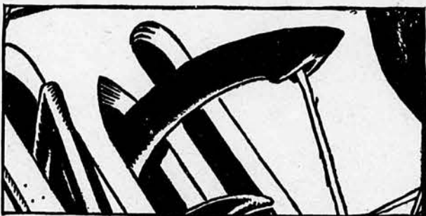
The needle — where "tow" bunches will catch and tangle.
