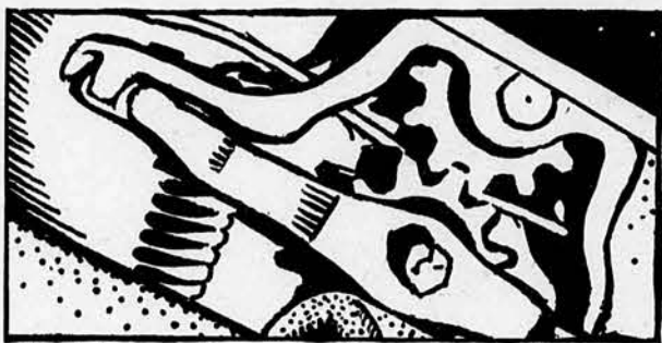
The tightener — here twine with weak spots often breaks
