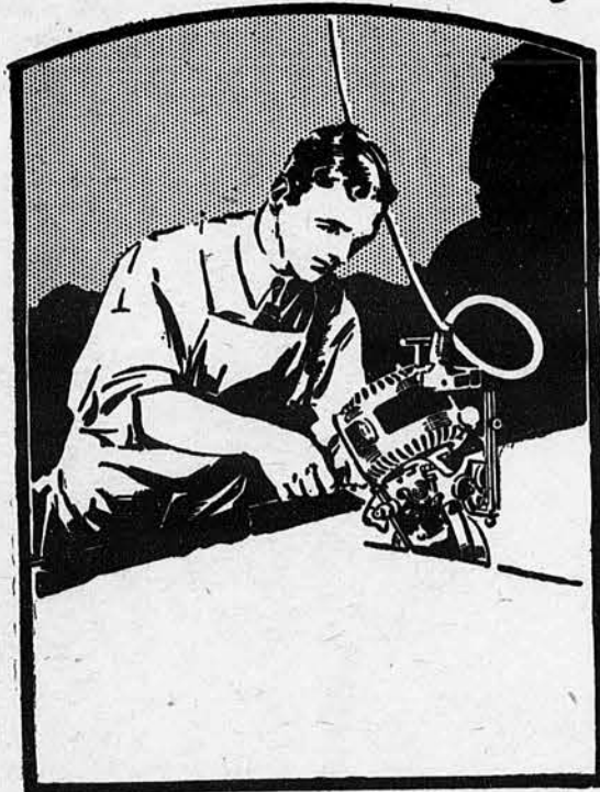
The electric knife used in cutting upholstery material for the Fisher Bodies, cuts 100 pieces of fabric at one operation as precisely and as quickly as one piece was formerly cut under methods which have been superseded by the new and more efficient Fisher methods
