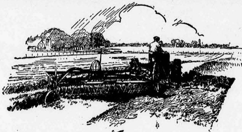
AT LEFT: Mowing and raking alfalfa in one operation with the Farmall, 7-ft. Farmall mower, and combined side rake and tedder. An ideal combination for speeding up operations and improving hay quality.
