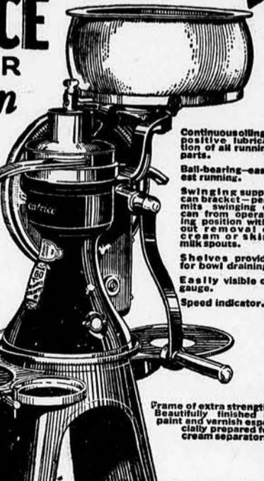
Continuous oiling—positive lubrication of all running parts.
