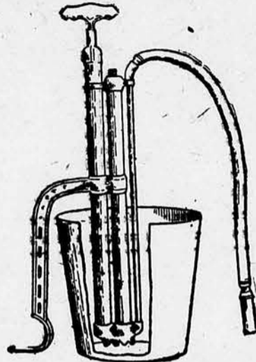
A Bucket Spray Pump Such as is Used in the Garden is Just the Thing to Spray the Poultry House
