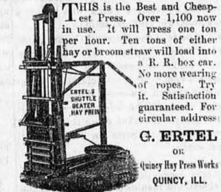
THIS IS the Best and Cheapest Press. Over 1,100 now in use. It will press one ton per hour. Ten tons of either hay or broom straw will load into a R. R. box car. No more wearing of ropes. Try it. Satisfaction guaranteed. For circular address: G. ERTEL, Quincy Hay Press Works, QUINCY, ILL.
