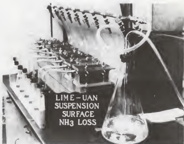
Figure 1. LABORATORY APPARATUS FOR TRAPPING AMMONIA LOST FROM LIME MATERIAL - UAN SUSPENSIONS
