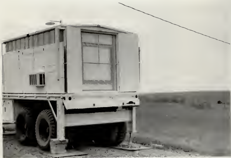
Plate 5. Rear of detector trailer showing collimator opening and trailer leveling system.
