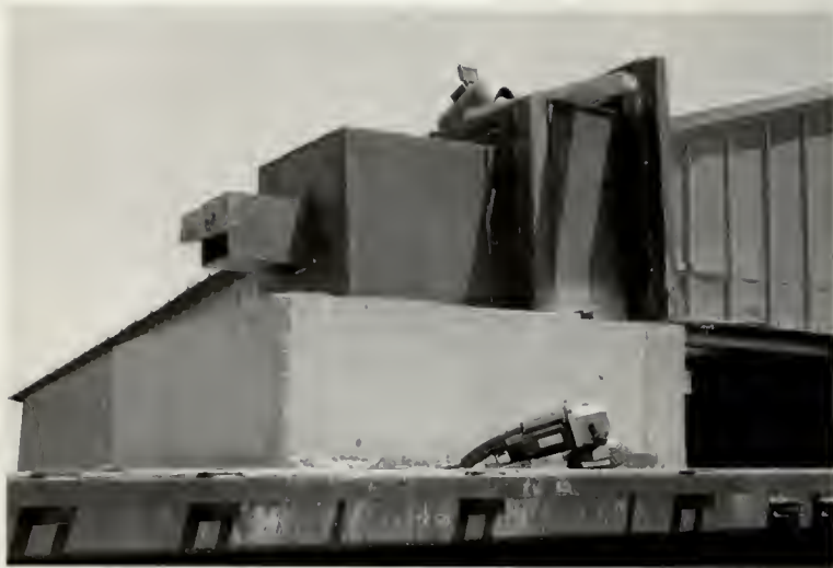
Plate 2. Unshielded detector cavity/collimator assembly.
