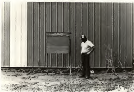
Figure 7. Plywood Box Housing the Controllers and Transmitters.
