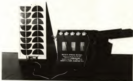
Figure 4. Ni-Cad Battery Used to Power the Receiver and Servos and Solar Panel for Re-charging the Battery.
