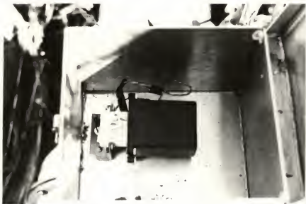
Figure 19. Modified Servo Mounted in Flow Control Valve Box.
