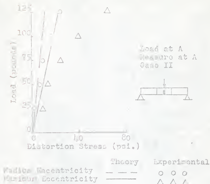
Fig. 24.-Load Vs. Distortion Stress at Lower Gage Location.
