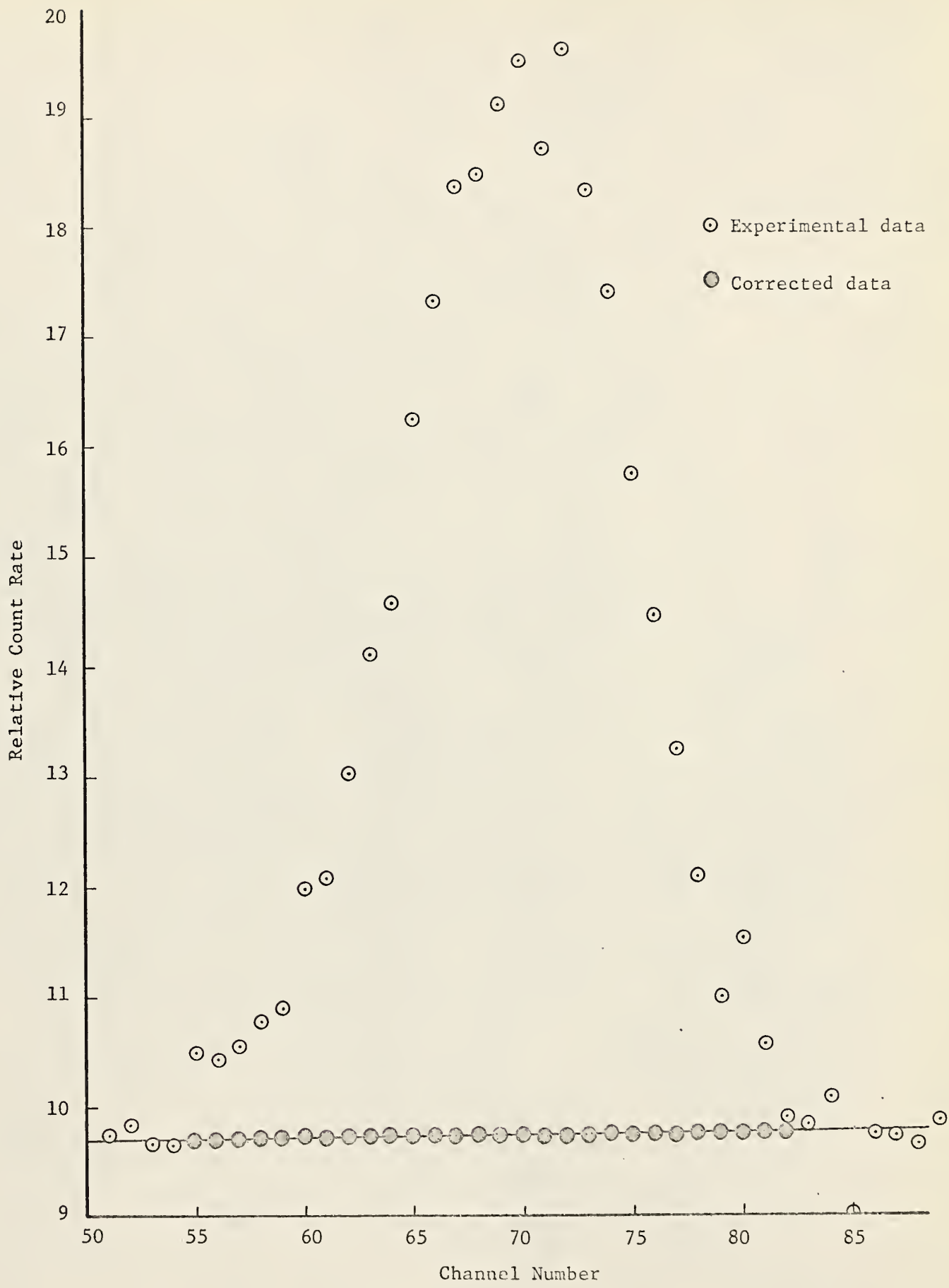
Figure 21. Illustration of spectrum correction technique, Hg-203 backscatter peak.
