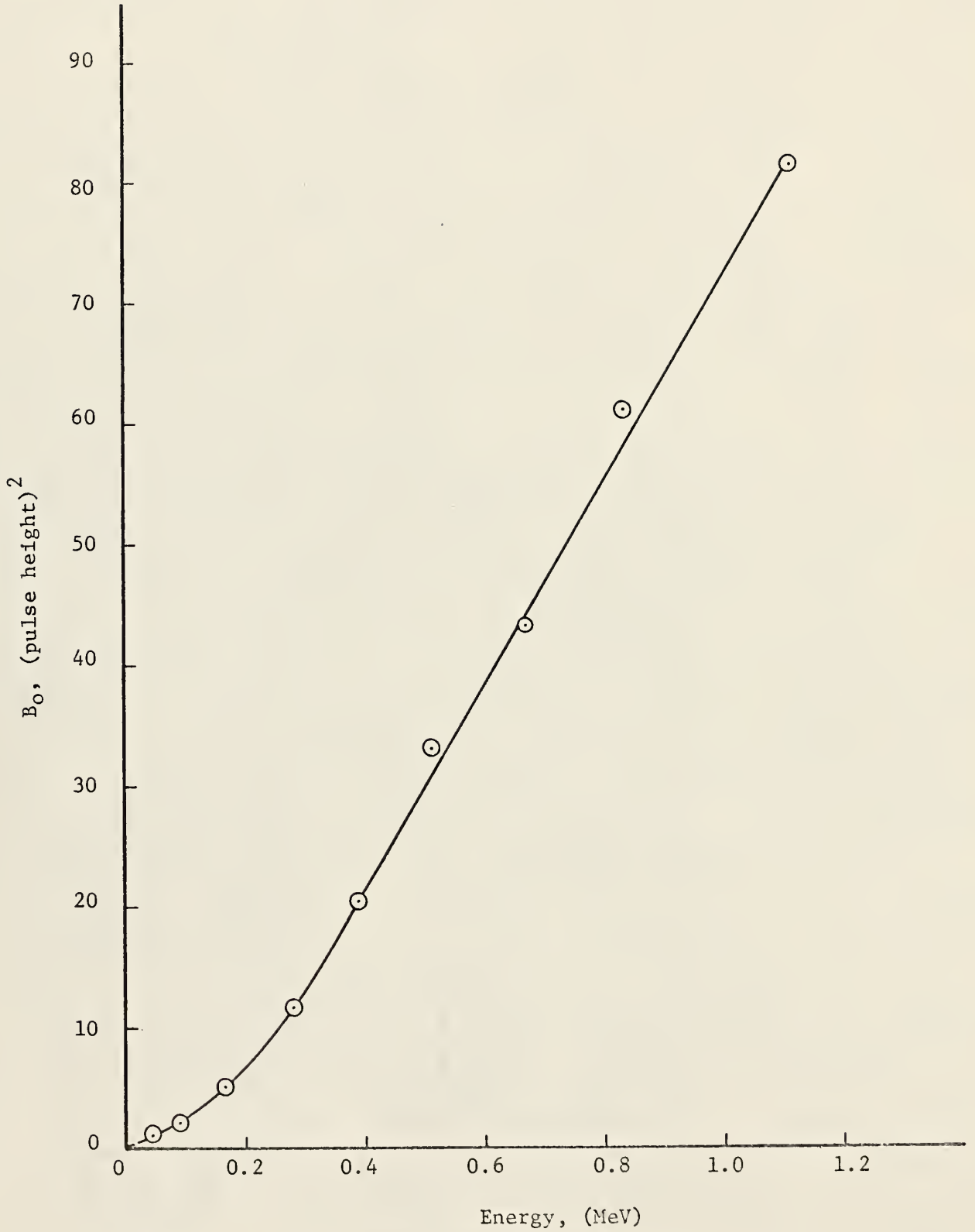
Figure 13. B_0 as a function of energy for two-inch collimator response functions.
