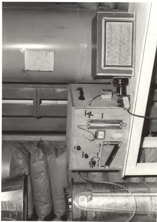
Figure 11. Cyclone discharge sampling system
