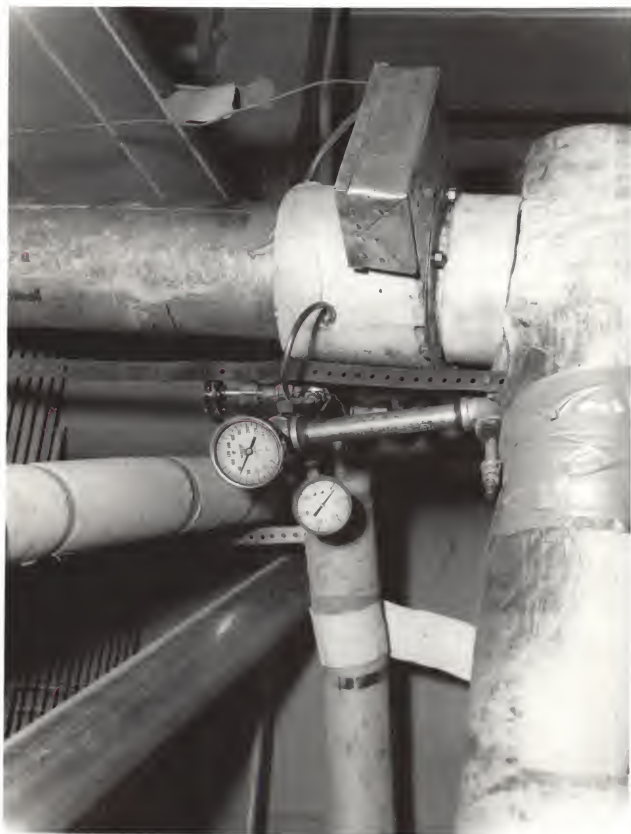
Figure 14. Liquid fat injector and screw conveyor
