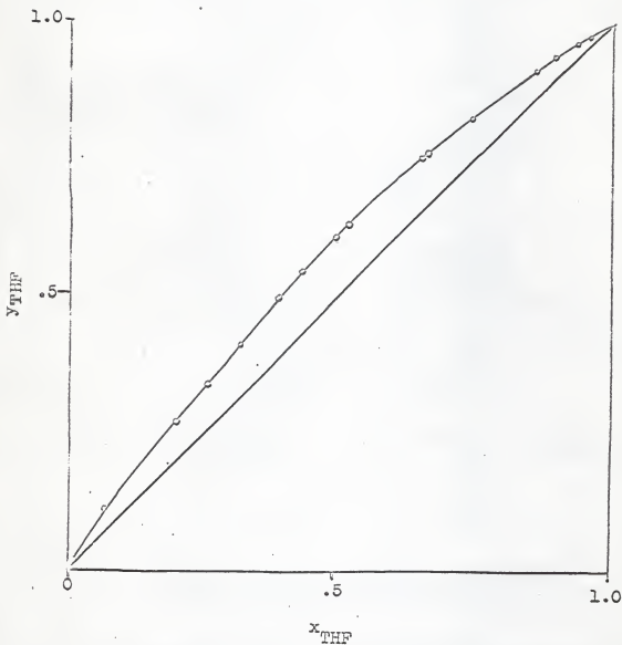
Fig. 3. Mole fraction THF in liquid versus mole fraction in vapor at 760mm. pressure, Benzene - THF.
