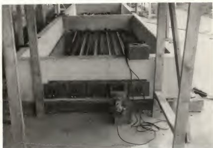
Fig. 14. View of tensioning bulkhead along with jack and Baldwin SR-4 strain indicator.
