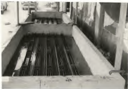
Fig. 15. View of bed just prior to molding test specimens. Bed has a capacity of 40 beams and 72 cylinders.
