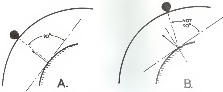
Figure 1 Illustrating that echoes can be detected from tissue interfaces only if the sound beam crosses the interface at right angles as in (A). At other angles of incidence (B), the echo does not return to the probe.
