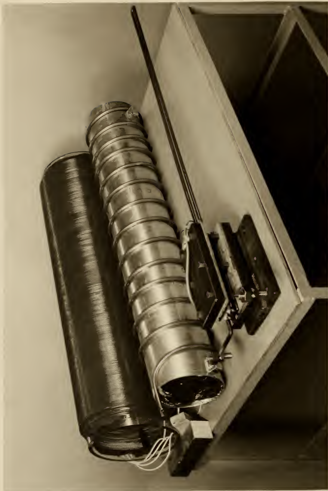
Figure 5. Field Coil, Heat Shield, Support, and Specimen.
