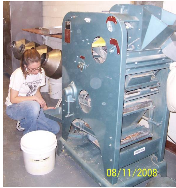
Figure 3.3 Left, Forster Lab Scourer. Right, Carter-Day Dockage tester.
