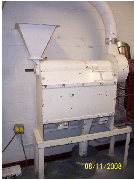
Figure 3.3 Left, Forster Lab Scourer. Right, Carter-Day Dockage tester.
