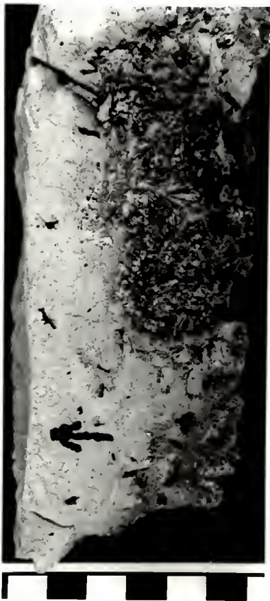
Figure 63. Nodular accumulation of chert filled rosettes, from the top of unit 11, locality GY 1. Scale in centimeters.
