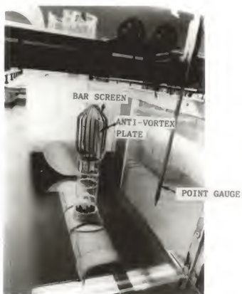
Figure 6. Side View of Open-riser with Bar Screen and Anti-vortex Plate installed in Flume
