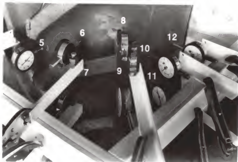
Figure 10. Photograph showing the actual location and numbering order of dial indicators 5-12.
