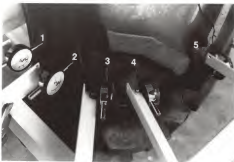
Figure 9. Photograph showing the actual location and numbering order of dial indicators 1-5.
