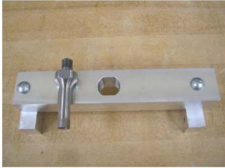
Fig. 8. Position of tool holding for observation of tool lateral face.
