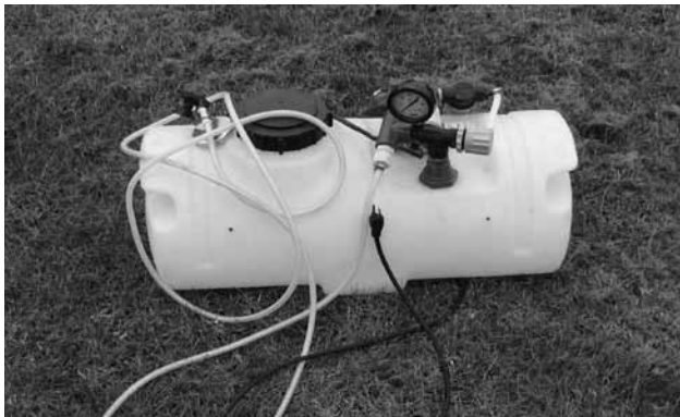
Figure 1. Small tank sprayer for applying grain protectants (photo courtesy of F. H. Arthur, USDA-ARS-CGAHR).
