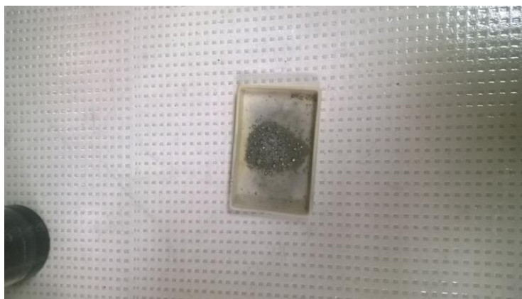
Figure 41 Ceramic boat after material removal after pyrolysis
