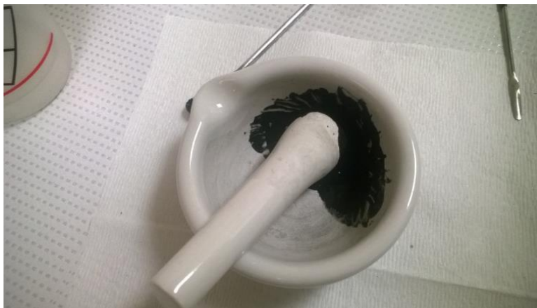
Figure 43 Mixing the pyrolyzed material with binder
