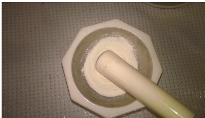
Figure 37 Crushed mixture to be put in for pyrolysis
