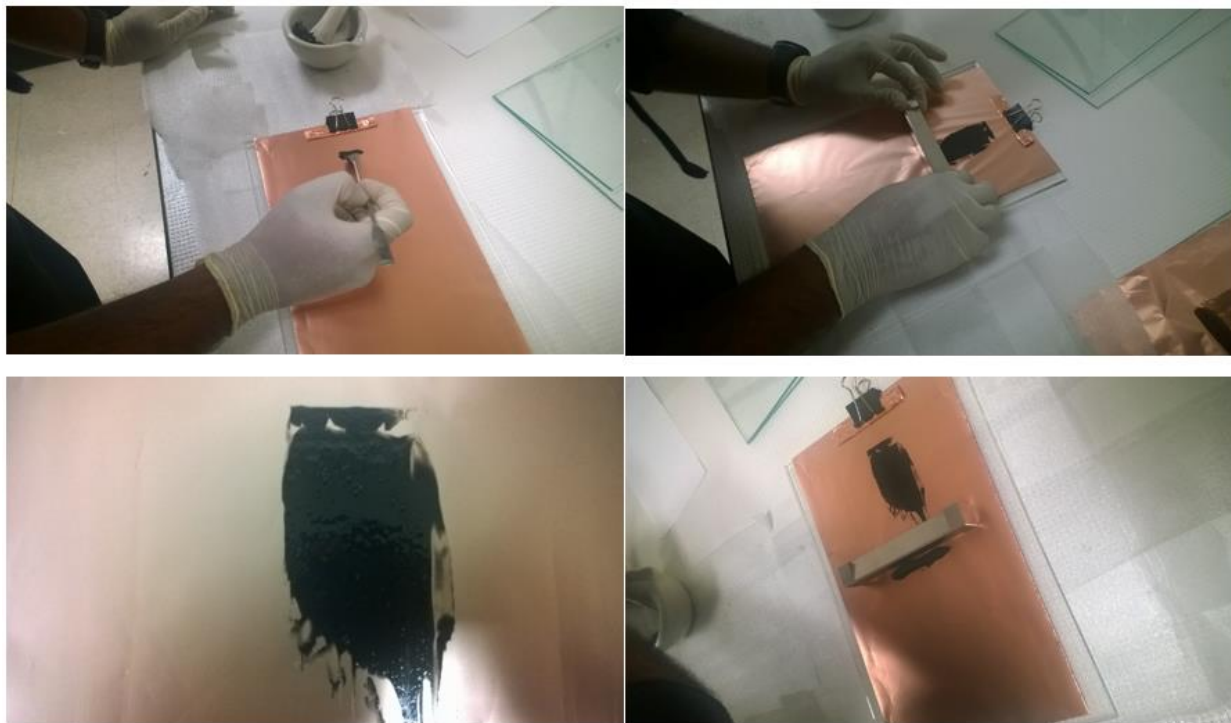
Figure 45 Coating the copper foil using the doctor blade method
