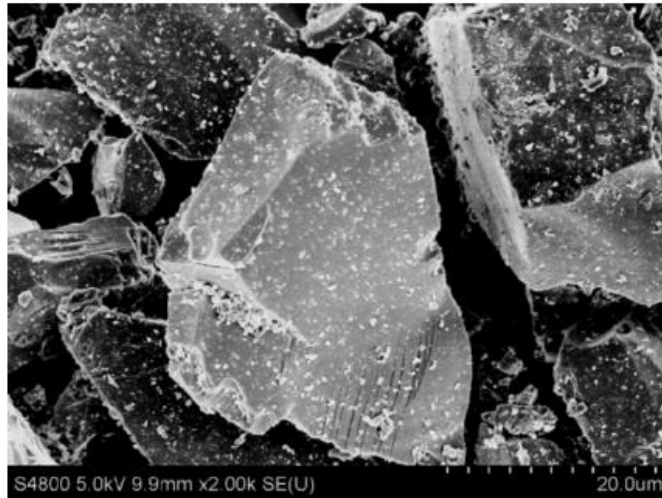
Figure 30 SEM image of the Si-O-C composite under a hydrogen atmosphere [57]
