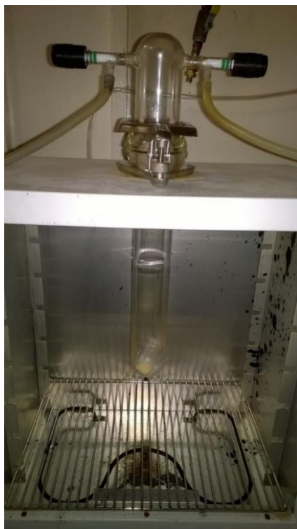
Figure 36 Showing the input and output gas pipes in the cross linking apparatus
