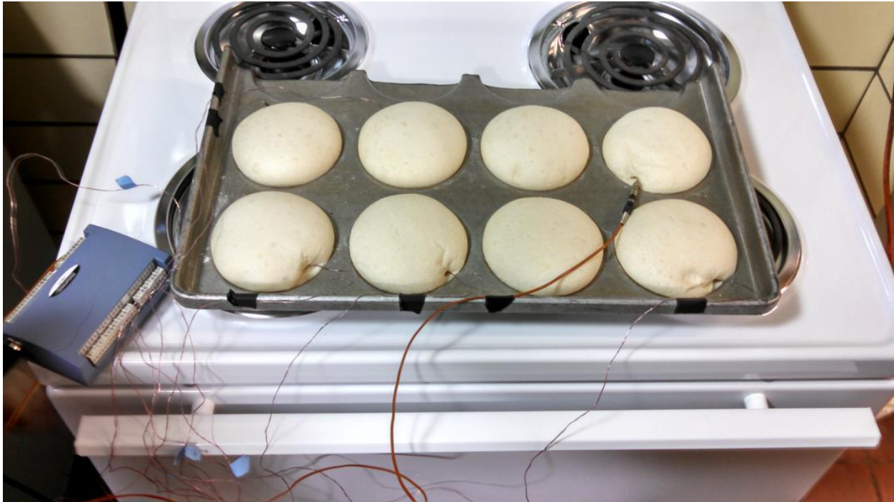
Figure A.6 Thermocouples were inserted into the geometric center of buns and one thermocouple was affixed to the side of the pan to monitor oven air temperature
