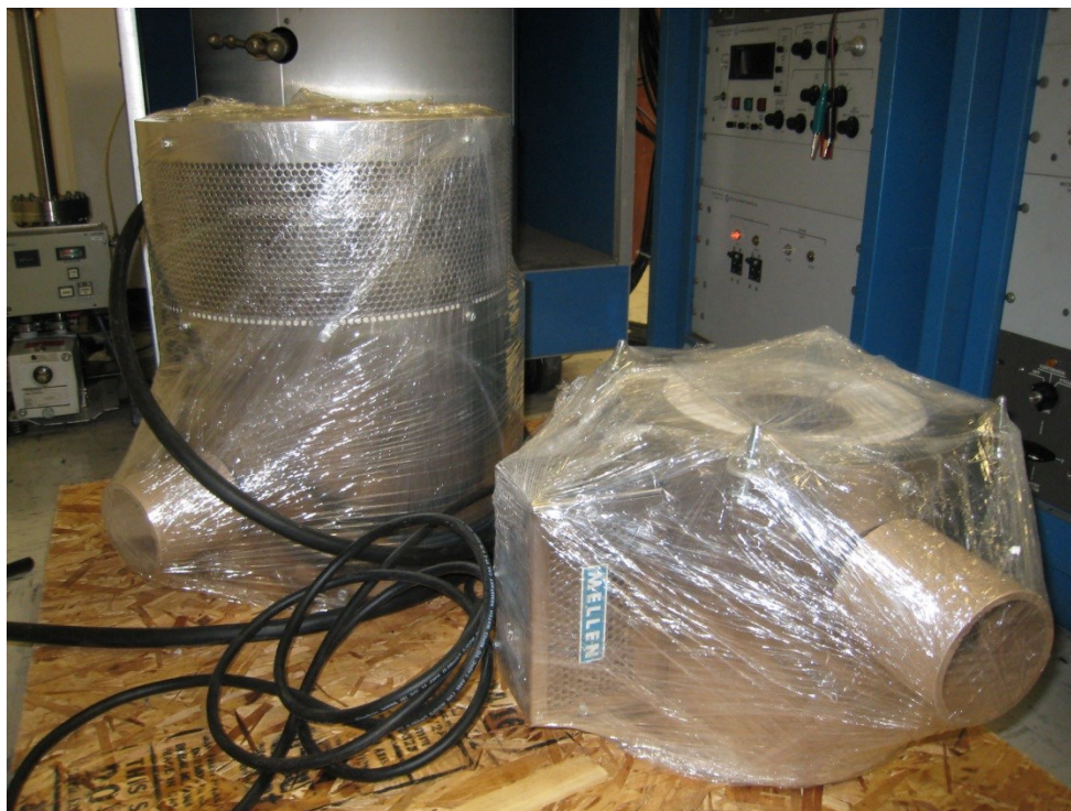
Fig. 4.8. The furnace zone components for the two-zone furnace as provided by Mellen Furnace Company. The 1500 °C zone (hot zone) is on the left, and the 1200 °C zone (cold zone) is on the right.
