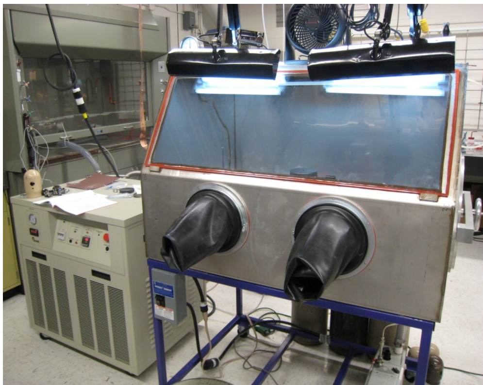
Fig. 4.28. The completed high-temperature glove box, equipped with an industrial chiller, cabinet lights, electrical breakers, and gas inputs / outputs.
