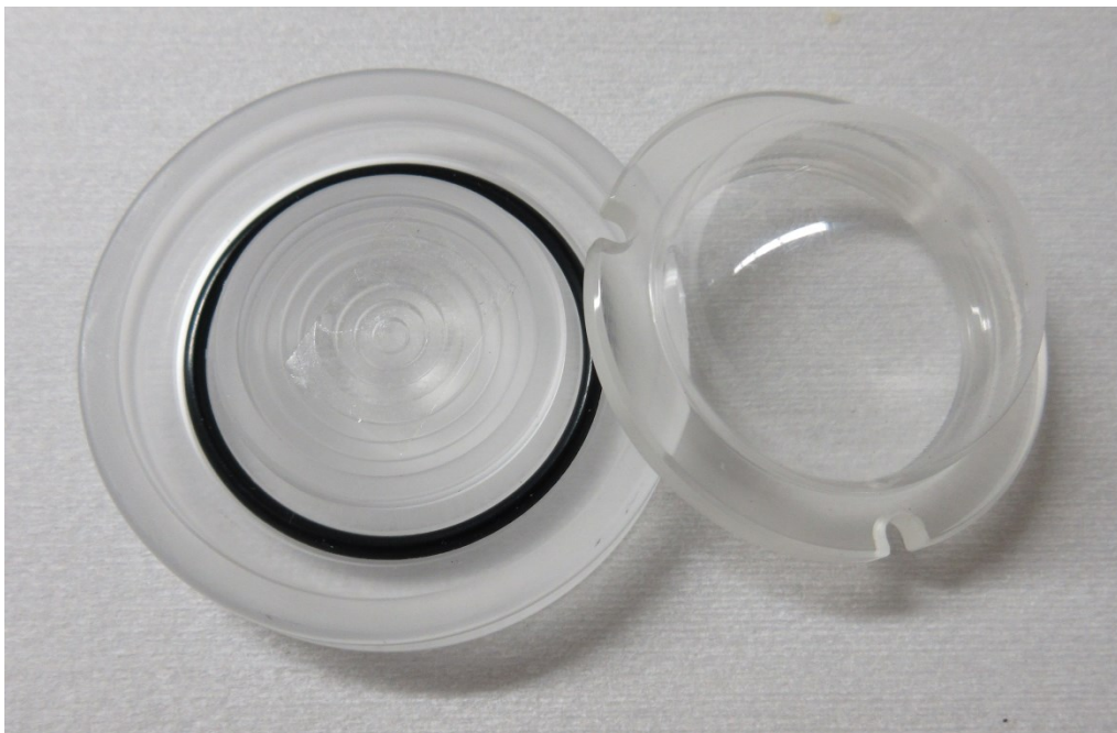
Fig. 5.38. Air-tight sample holder provided by Bruker AXS Inc. The PMMA plastic base with double-sided sticky tape (left) and the beryllium dome (right) that screws firmly to the o-ring seal on the base.
