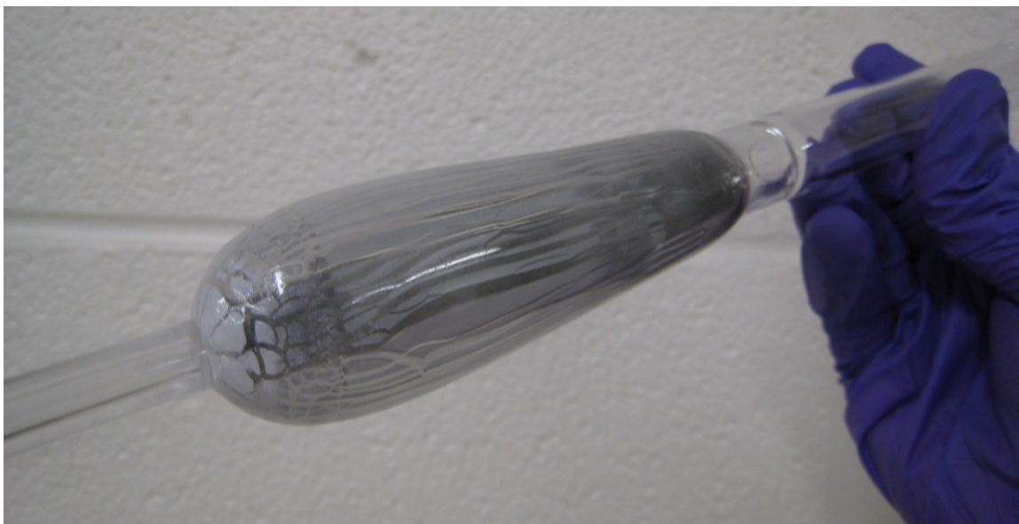
Fig. 4.38. An example of a vacuum sealed ampoule, containing a high vapor pressure material that was ramped in temperature to >1100^{\circ}\text{C} .
