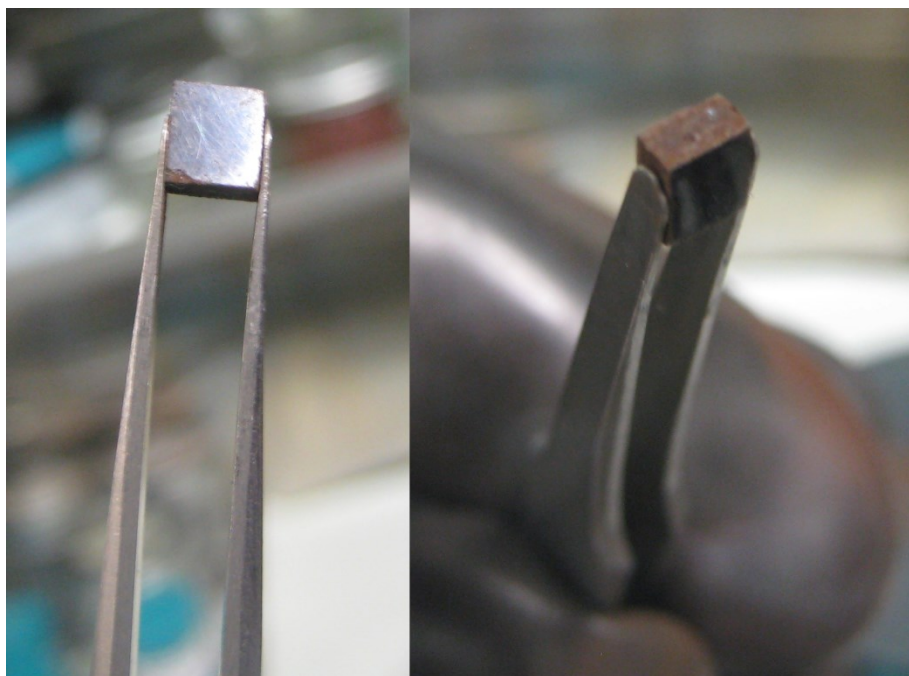
Fig. 5.36. A 4.077 \times 3.518 \times 2.020 \text{ mm}^3 bulk grown crystal of purified LiZnP.
