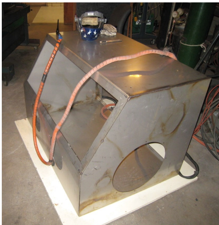
Fig. 4.25. The welded glove box
