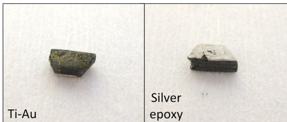
Fig. 6.48. A LiZnP sample with a silver epoxy (cathode) contact and a 500 Å / 10,000 Å Ti/Au gold (anode) contact. This is the same sample with the I-V response shown in Fig. 6.15 with approximate dimensions 2.0 x 3.0 x 5.0 mm 3 .
