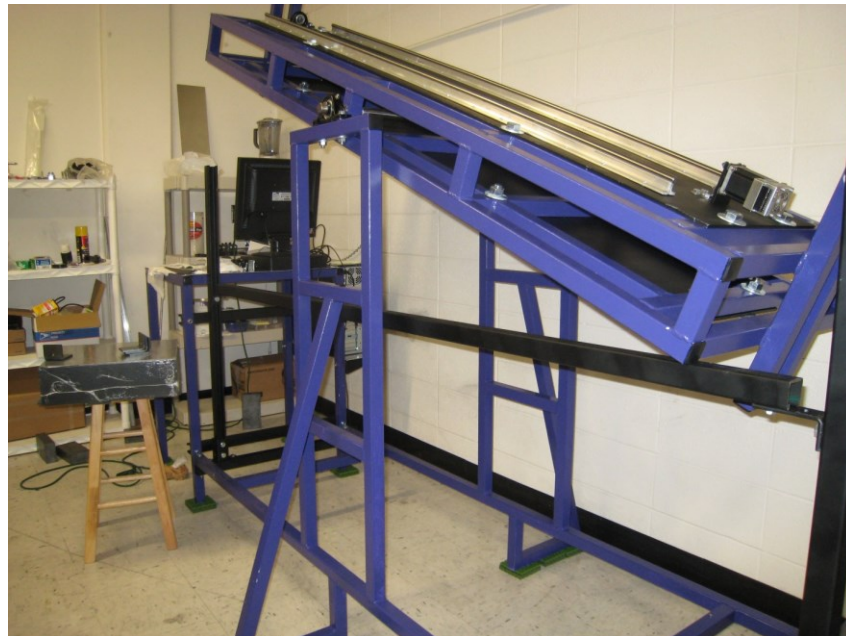
Fig. 4.6. The furnace frame with the rotation table, and mounting plates installed.
