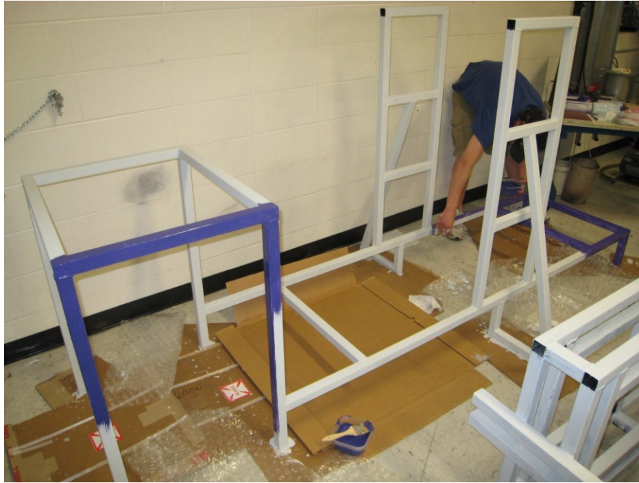
Fig. 4.5. Furnace frame in the painting process.
