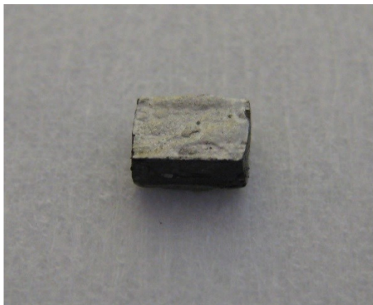
Fig. 6.3. A LiZnP sample with a silver epoxy contacts on two sides with HumiSeal® encapsulating the remaining sides
