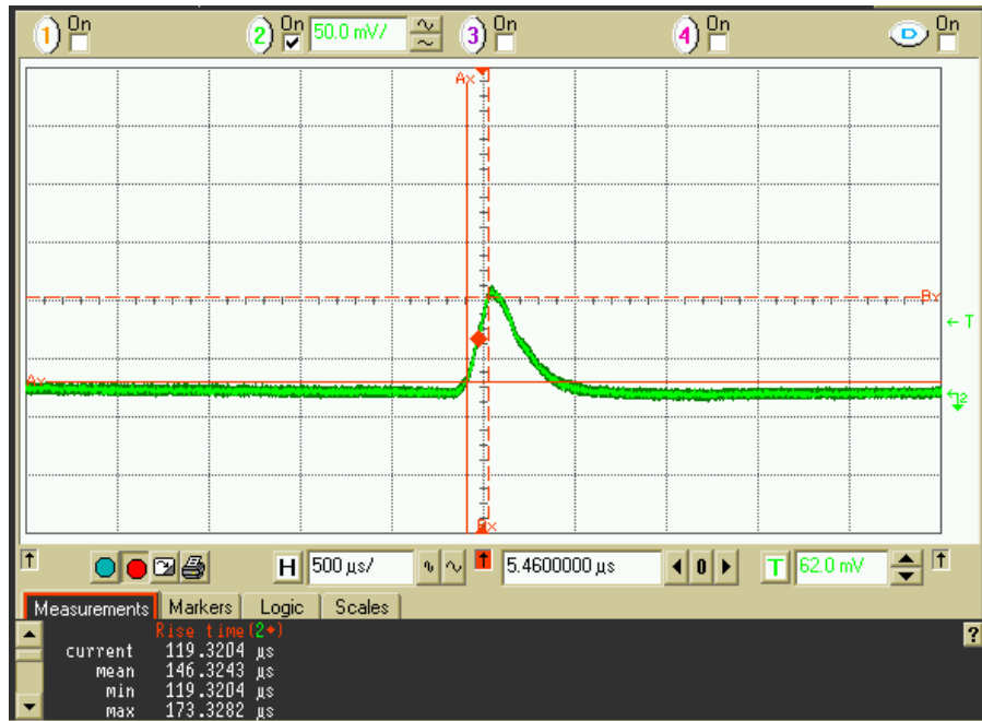
Fig. 6.33. The resulting signal from 5.48MeV alpha partial absorption from cathode irradiation in LiZnAs sample.
