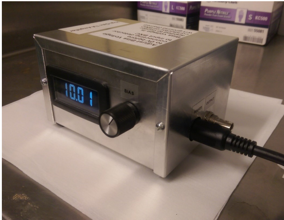
Fig. 6.44. Custom electronics package for the high-gain trans-impedance amplifier (TIA) designed and fabricated by the Electronics Design Laboratory (EDL) of Kansas State University.
