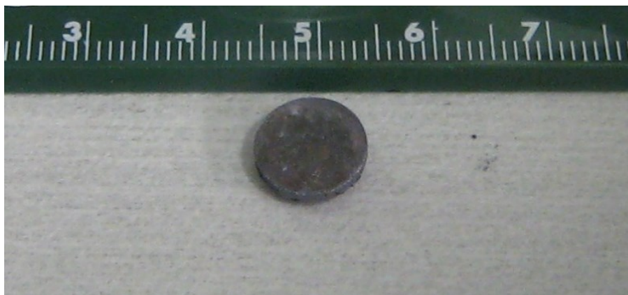
Fig. 5.35. Slice from the LiZnP purified ingot (picture collected through the glove box window).
