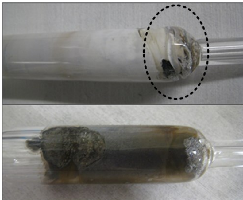
Fig. 5.4. Example of ampoule cracking (circled portion) (top), and example of a successful ternary material synthesis using a graphite crucible (bottom).
