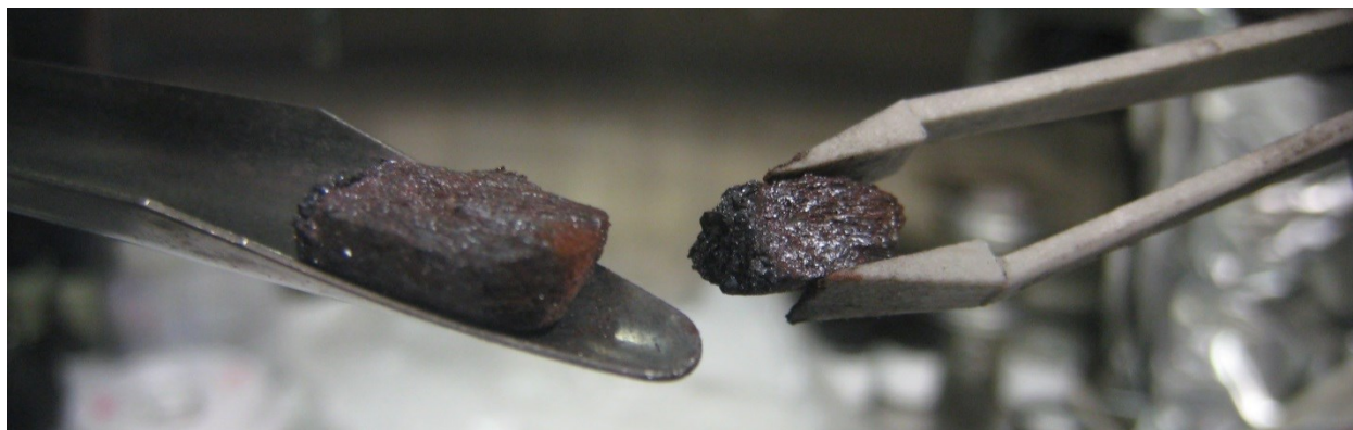
Fig. 5.32. LiZnP crystals grown by the high-temperature growth method (picture collected through the glove box window).
