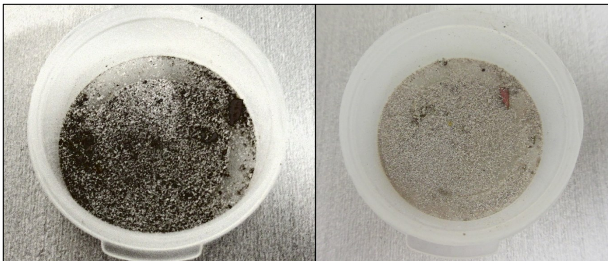
Fig. 6.5. The repolished LiZnP sample after 1 month (left) of exposure to air, and after >2months (right) of exposure to air.
