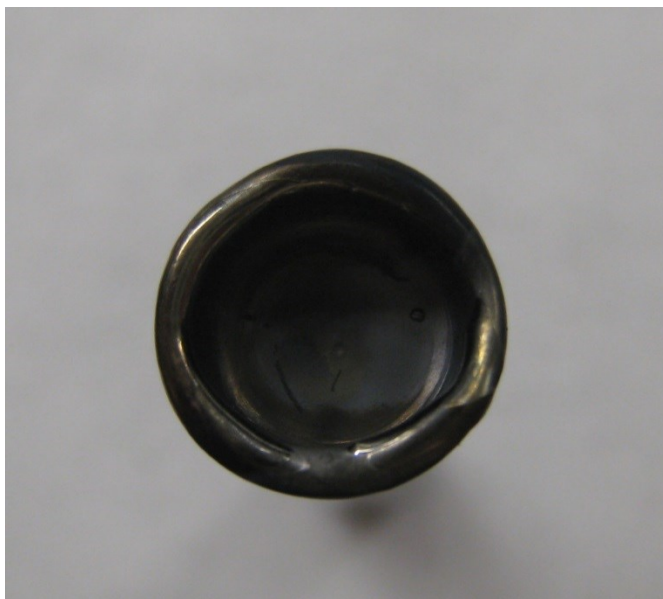
Fig. 5.25. A view of the arc-welded tantalum cap that makes a pressure-tight seal.
