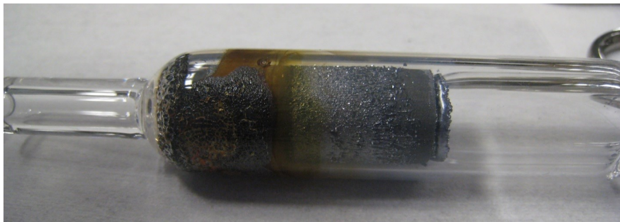
Fig. 4.39. The resulting LiZnAs reaction / synthesis process ampoule. Reaction with the quartz is seen by the dark coloration on the quartz wall, and crystallization on the outside of the ampoule was observed.
