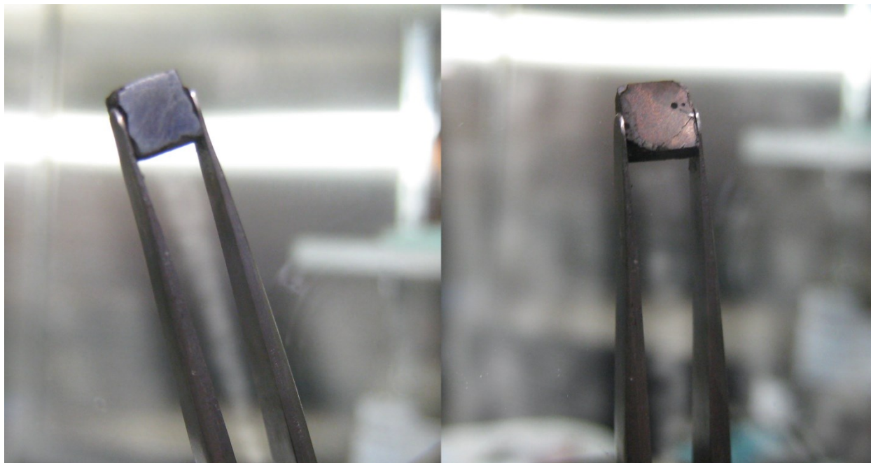
Fig. 5.46. Both sides of a LiZnAs sample, the sample used for x-ray diffraction analysis with dimensions of 2.100 \times 4.060 \times 4.155 \text{ mm}^3 .
