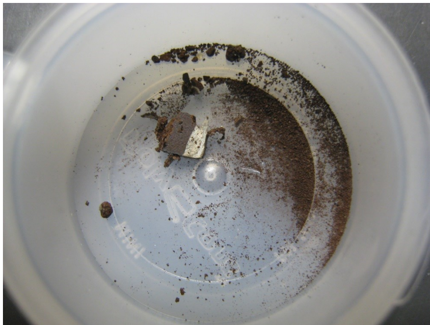
Fig. 6.4. The repolished LiZnP sample after approximately 48 hours of exposure to air.
