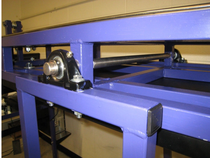
Fig. 4.7. A detailed look at the pillow block, and the rotation table design for vertical, horizontal, or tilted crystal growth.
