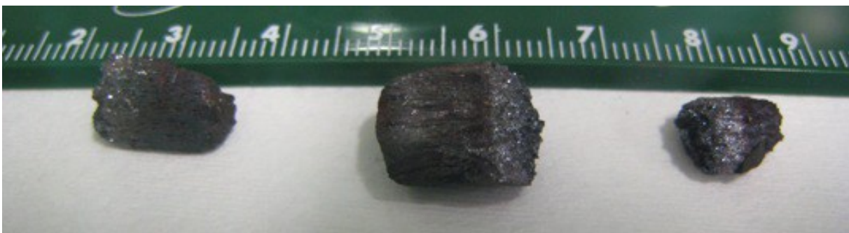
Fig. 5.31. LiZnP crystals grown by the high-temperature growth method (picture collected through the glove box window).
