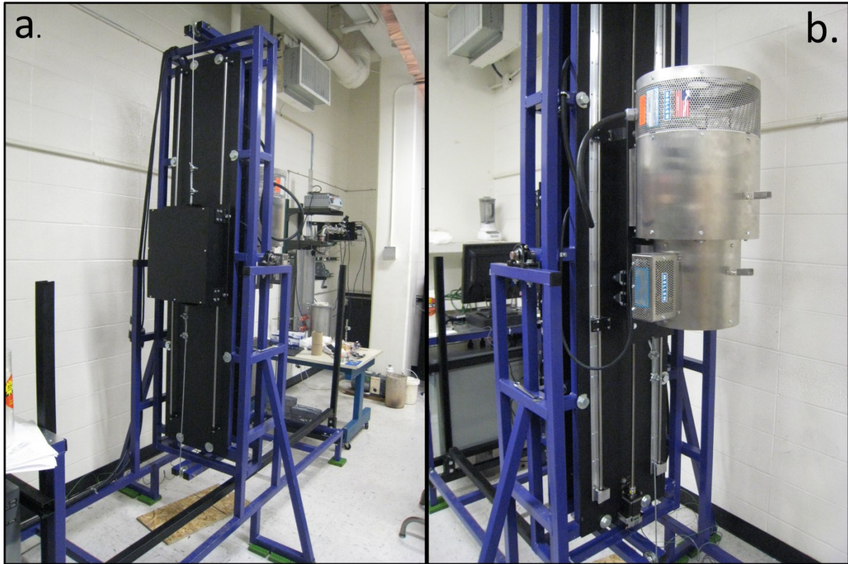
Fig. 4.9. a. A view of the completed crystal growth furnace, where the removable counter weight is shown. b. A view of the completed crystal growth furnace, where the furnace zones are shown in the vertical position
