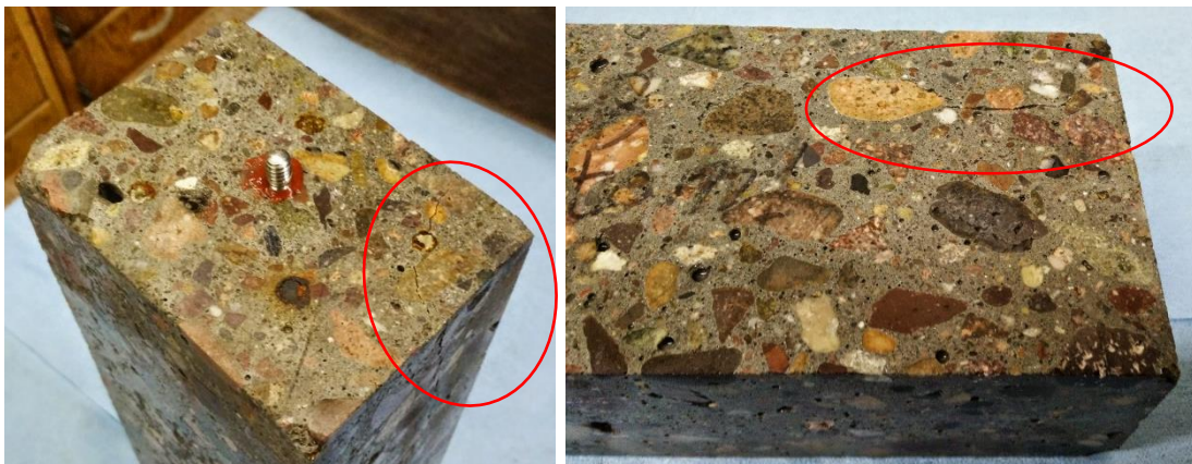
Figure 5.8 Cracking pattern in saw-cut samples in freeze-thaw testing (SHT3)
