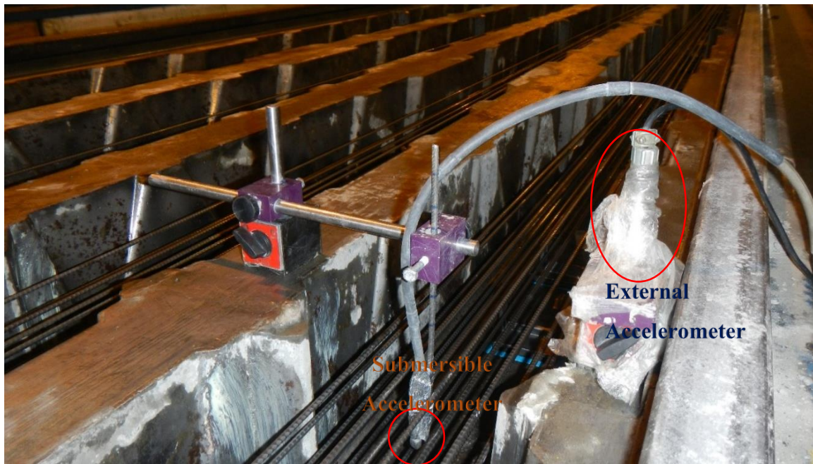
Figure 3.12 Two accelerometers in position for recording
