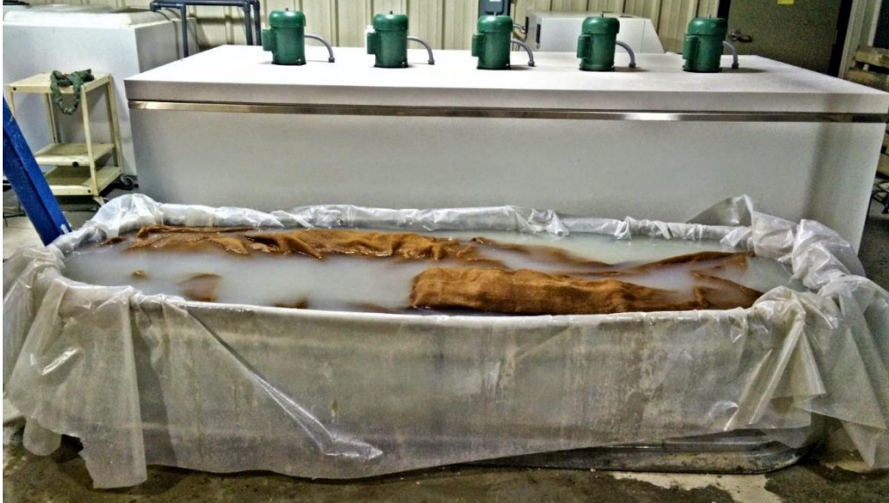
Figure 5.1 Soaked half ties covered with burlap
