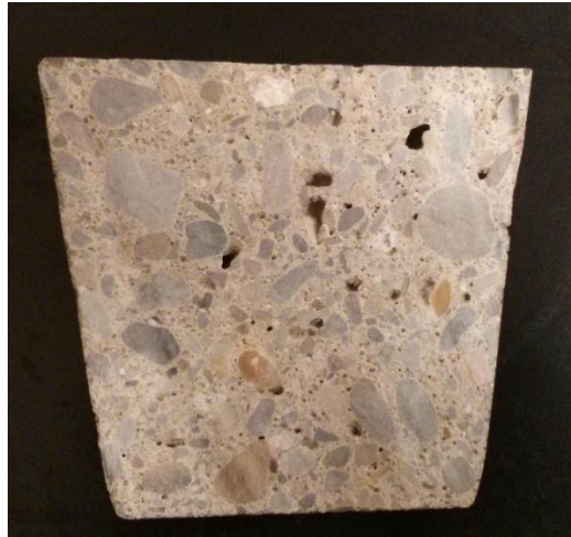
Figure 3.16 Hardened air void sample after cutting
