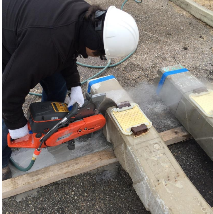
Figure 5.4 Saw-cutting samples from the tie end
