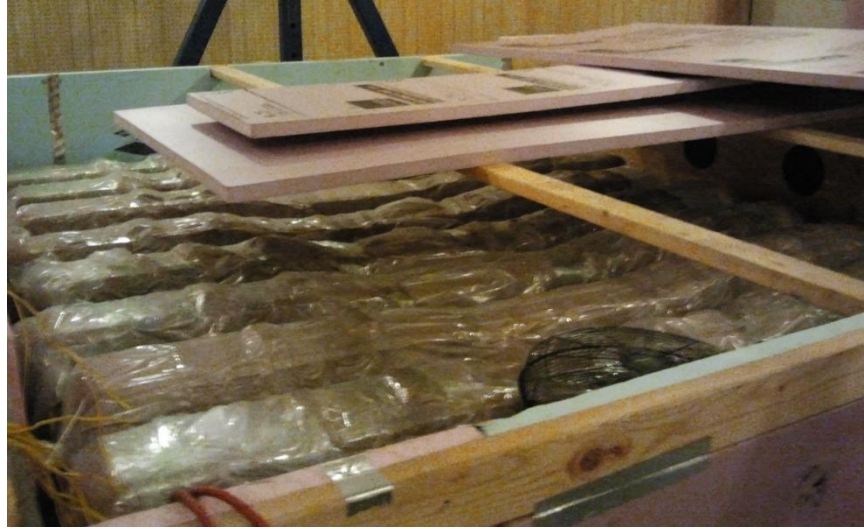
Figure 4.6 Railroad ties in the testing chamber
