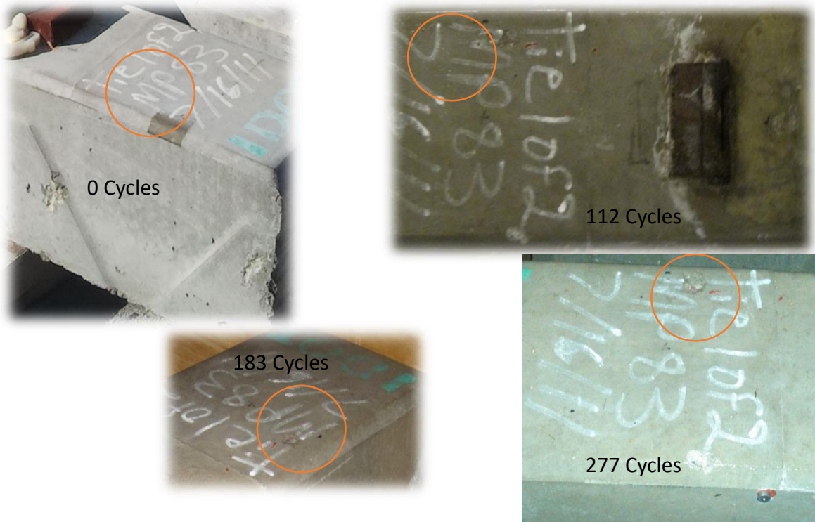
Figure A-24: Tie #1-05009-3 Plant C visual observations
