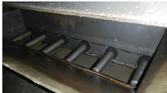
Figure 3.6 Plant A vibration rods attached to the casting machine
