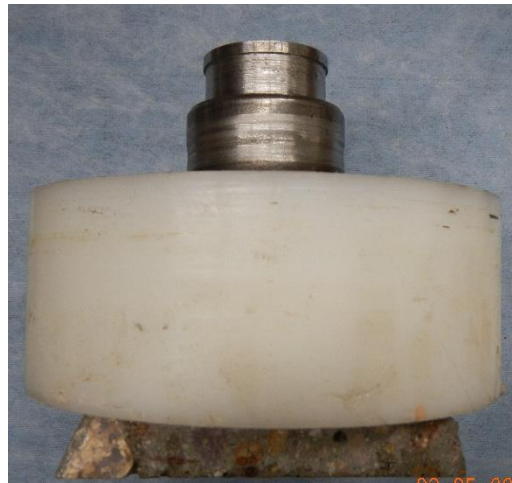
Figure 3.17 Side view of hardened air void sample attached to the rotation cylinder
