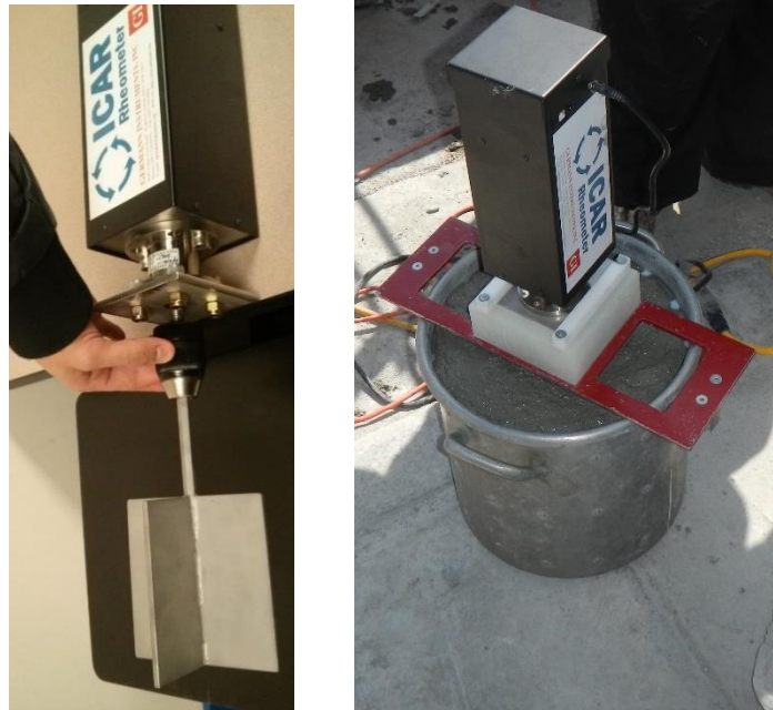
Figure 3.9 ICAR rheometer a) with the vane, and b) in use
