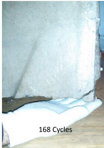
Figure 4.24 Tie #2-4386-B corner piece after fracture
