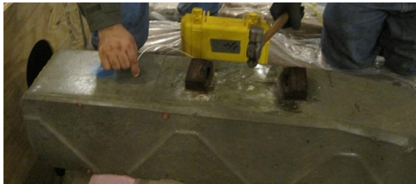
Figure 4.10 Resonant frequency measurements
