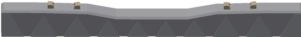
Figure 2.1 Typical prestressed concrete crosstie
