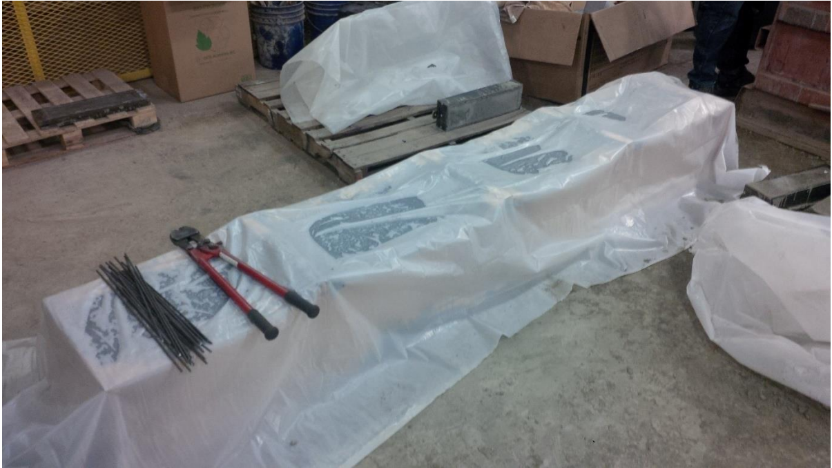
Figure 7.4 Unreinforced tie covered in plastic
