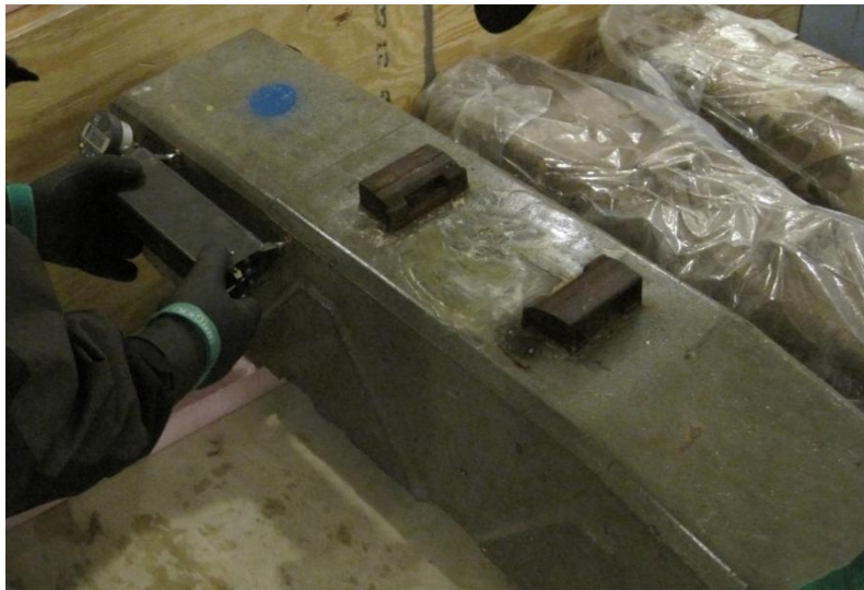
Figure 4.9 Whittemore point length measurements
