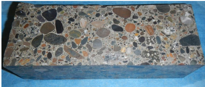
Figure 5.6 Typical 4 x 3 x 11 in. saw-cut freeze-thaw sample
