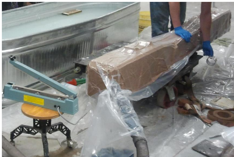
Figure 4.4 Railroad tie vacuum-sealed and wrapped with packing tape
