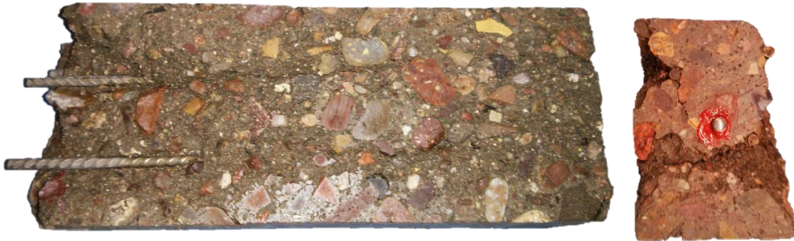
Figure 5.10 Mass loss for saw-cut samples in freeze-thaw testing (SHT4)
