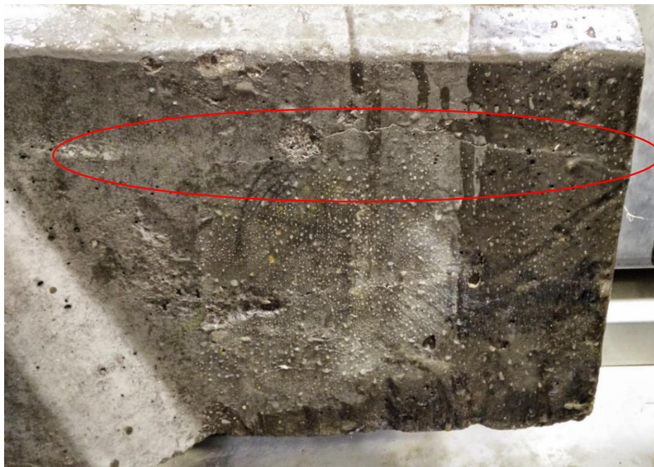
Figure 6.4 Half tie (HT4) crack appearance at 248 cycles of freeze-thaw
