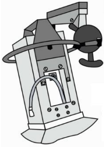
Figure 1. Waveguide applicator. Adapted from “Hyperthermia in combined treatment of cancer” by Wust, P., Hildebrandt, B., Sreenivasa, G., Rau, B., Gellermann, J., Riess, H., Felix, R., Schlag, P.M, 2002, The Lancet Oncology , 3, p.489.
