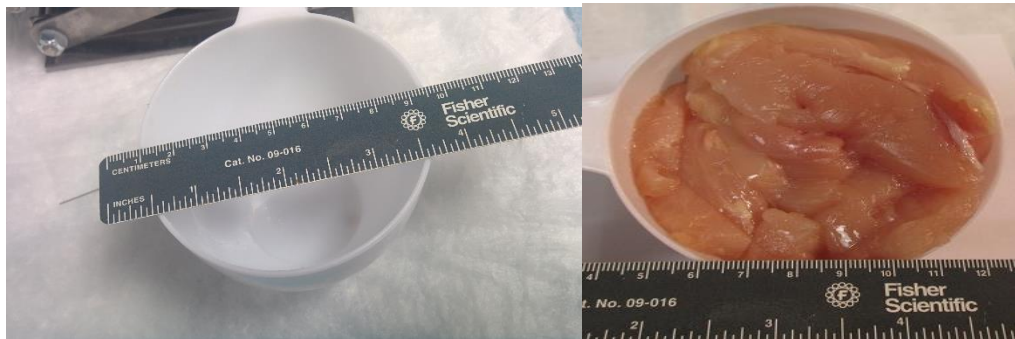
Figure 14. The breast model prepared by stacking meat in a hemispherical cup
