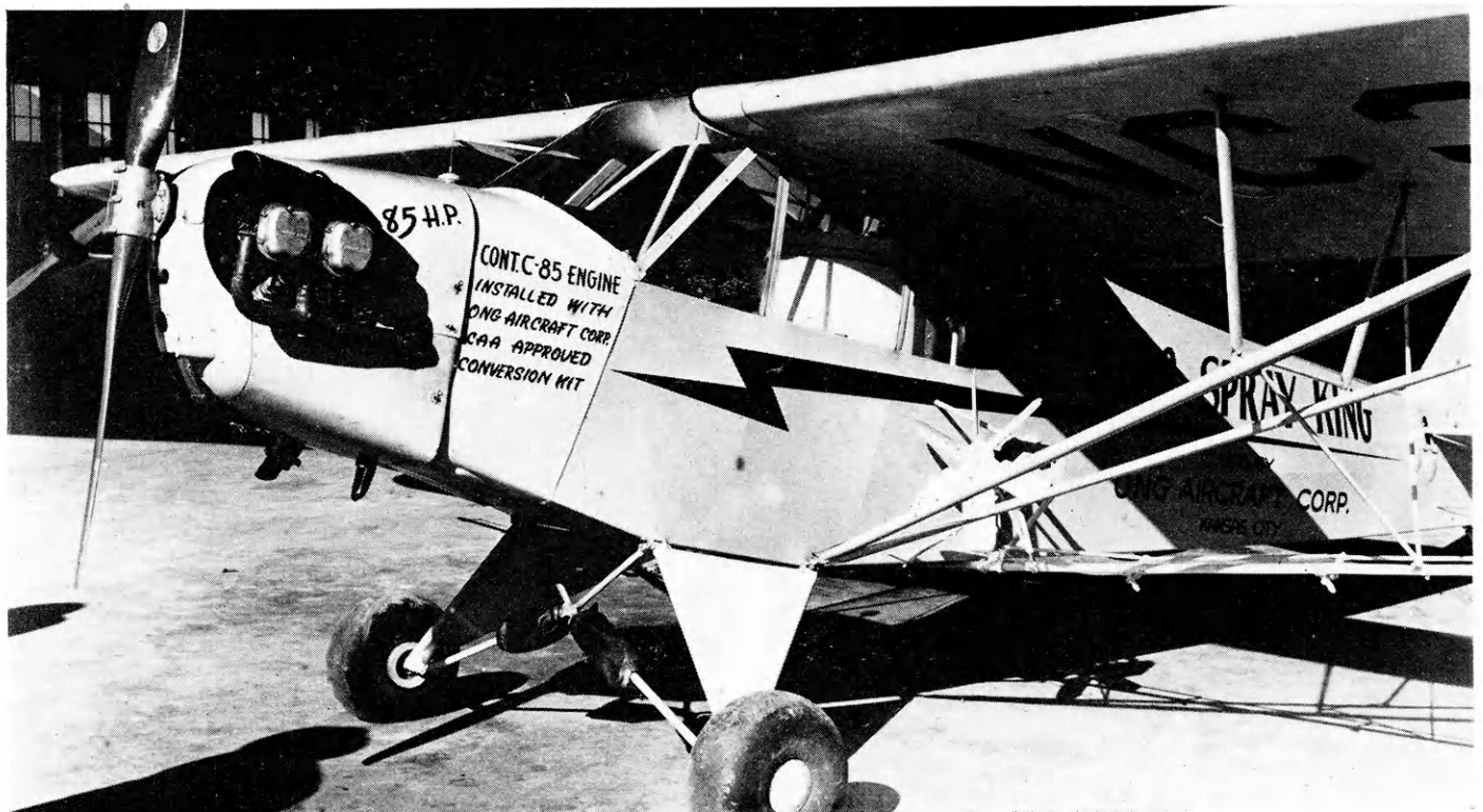
A slightly different installation on another Cub. Notice the tank in the rear seat, the spray boom below the struts, and another slipstream-driven pump fan. Photo by Jennings.
