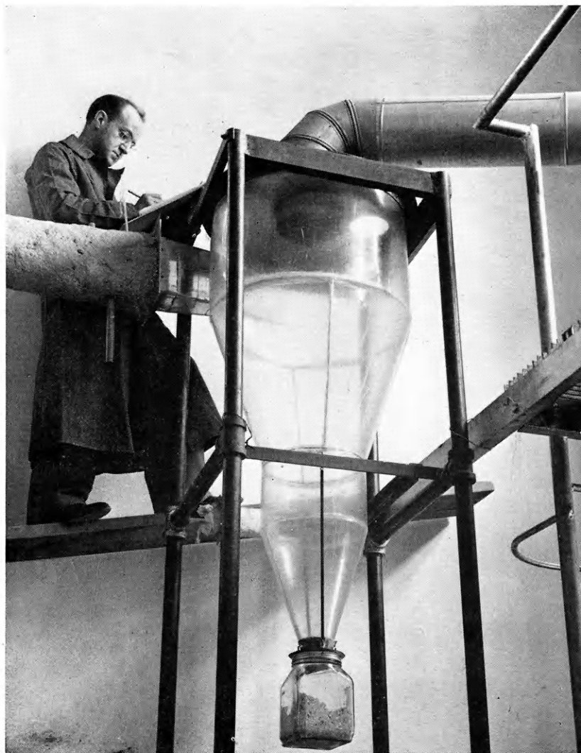
Allen L. Olsen records the results as the powder passes through a cyclone re-drier. This re-drier is a special model set up in the pilot plant here at Kansas State for the experiments recorded in Technical Bulletin 64.
