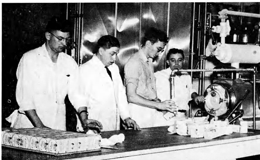
Making ice cream is now an assembly line proposition. Here Harold Eversmeyer, Gail Clemens, John Elam, and Val Zeigler demonstrate the ice cream making process in the new continuous freezer in the College dairy.
