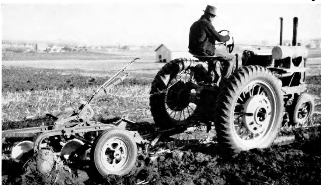
Testing a rubber tired tractor for fuel consumption, rolling resistance, and traction. The results of this test by the department of agricultural engineering can be used in determining the size of power unit needed on certain jobs.
