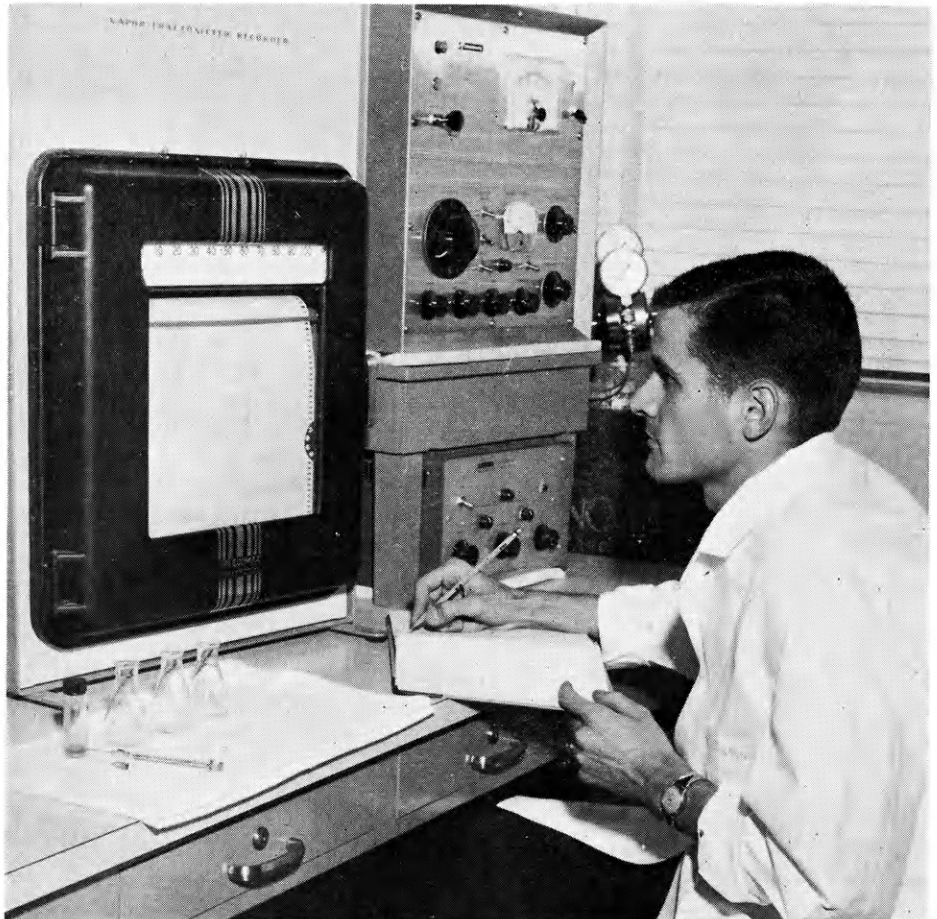
Richard Pylar of Chicago in a Kansas State University bakery management research laboratory measuring compounds that are responsible for bread flavor. K-State has done extensive research on both aroma and flavor of bread and other bakery products.
