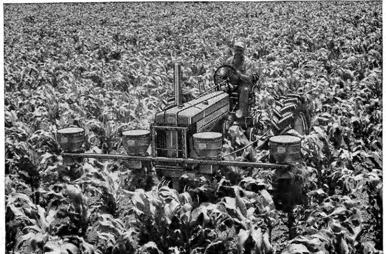
John Deere DDT Applicators are available in 4- and 6-row sizes. As the illustration shows, the John Deere Applicator is front-mounted to give the operator a good view of his work.
