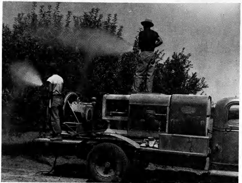
A MODERN power spraying set-up will do the job more efficiently and in much less time.
