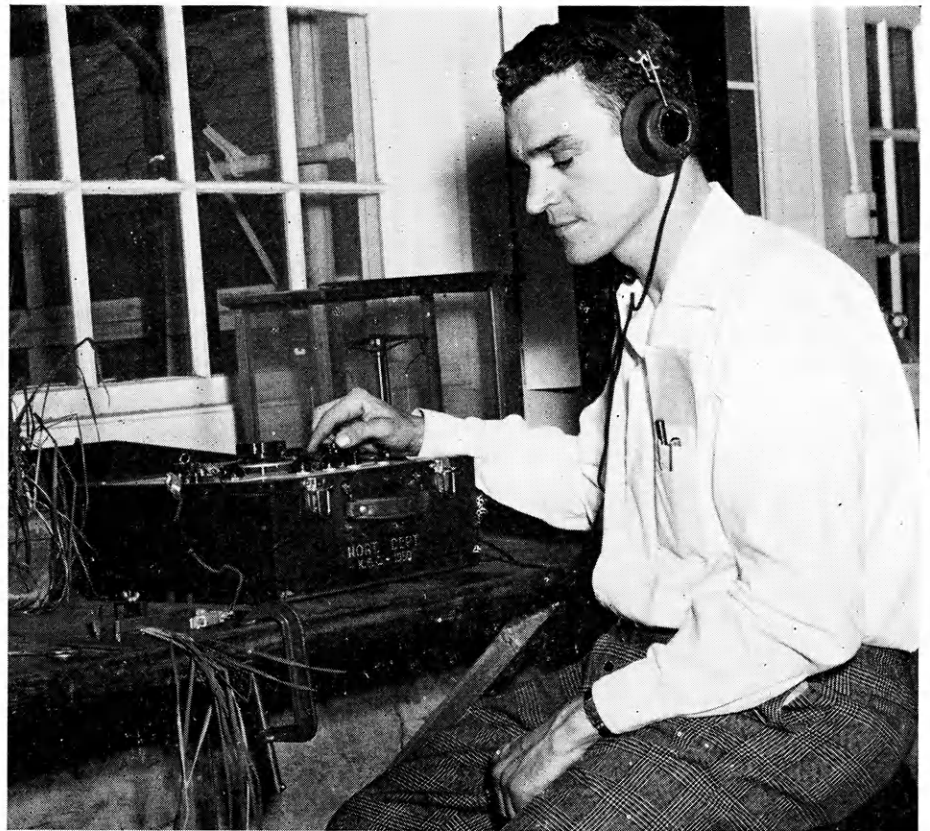
RESEARCH ASSISTANT BYRD CURTIS listens for the tone as he sends an electric current through a wheat stem. The experiment is designed to set-up a relation between electrical conductivity in a wheat stem, and hardness to heat, cold, and drouth.
